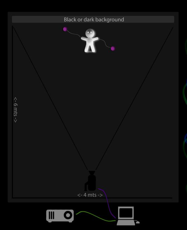
Because of Firewire cable length limitations, the computer must be placed not more than 10 mts. away from the camera. Having this in consideration, the VGA cable that connects the computer to the beamer/s must be long enough to reach the computer's location.
